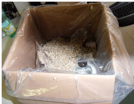
Details of an expedition of alcohol: samples contained in plastic bags are covered up by vermiculite
